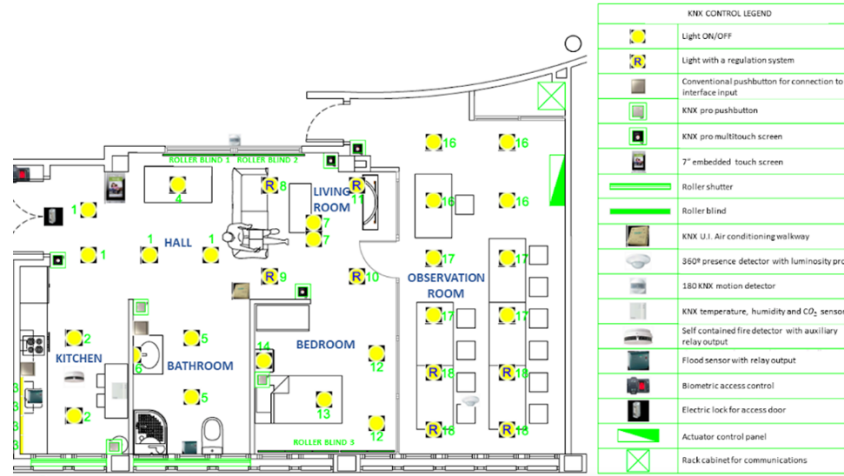
Fig. 3: Diagram of sensors and actuators in the Smart Home environment.
