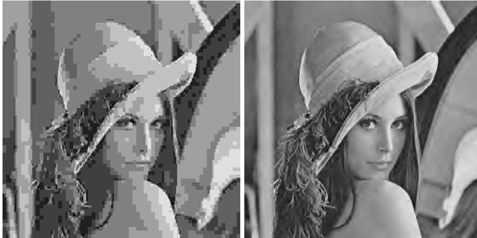
Figure 8: A JPEG-lossy (left) versus SPIHT (right) comparative for “lena” ( 512 \times 512 \times 8 ). The compression ratio is 0.14 bpp (51:1).
