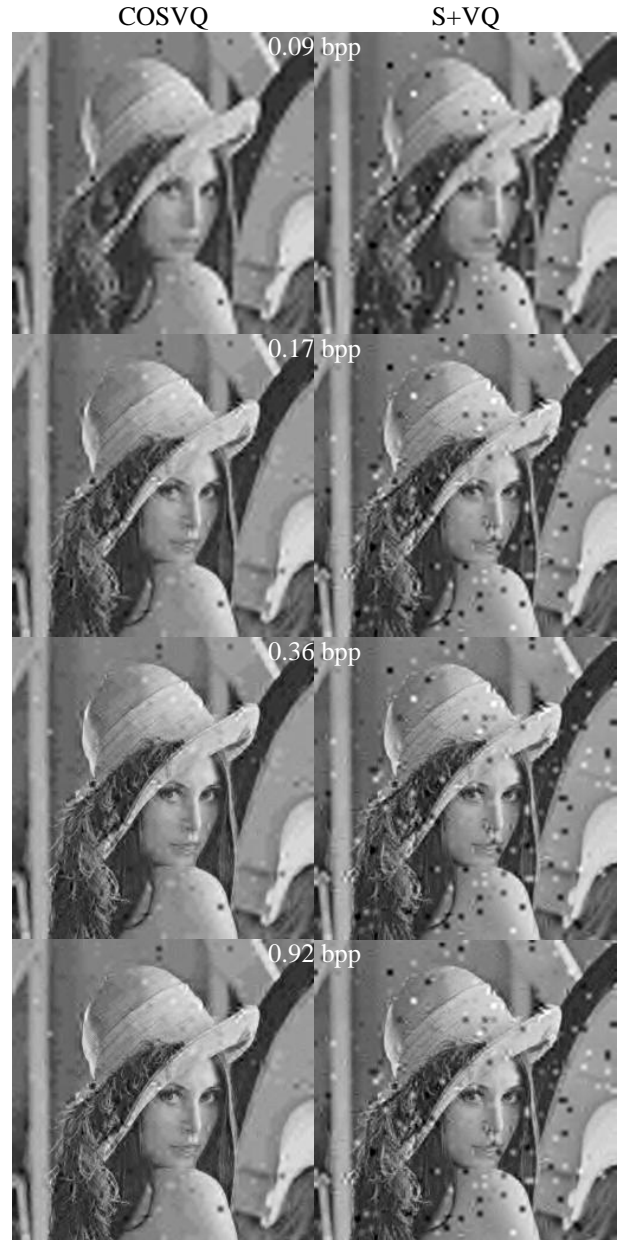
Fig. 3. Examples of progressive transmissions (AWGN Channel; CSNR = 6 dB).
